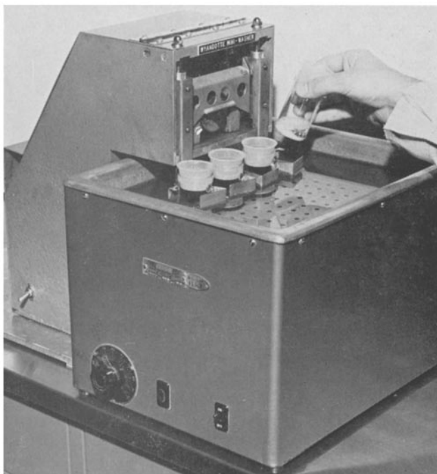
Fig. 1. Washing machine used in redeposition tests.
